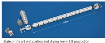
State of the art wet coating and drying line in LIB production
