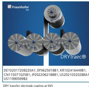
DRY transfer electrode coating at IWS
