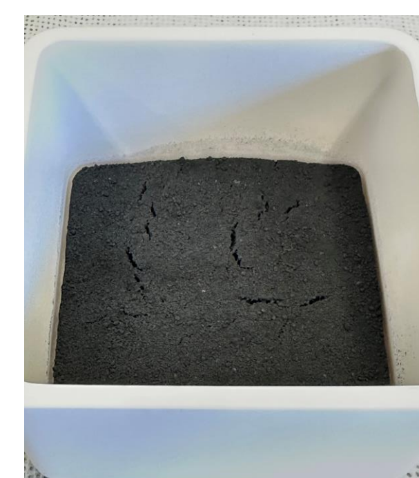
30 g calcined NNFM powder in an \text{Al}_2\text{O}_3 crucible
