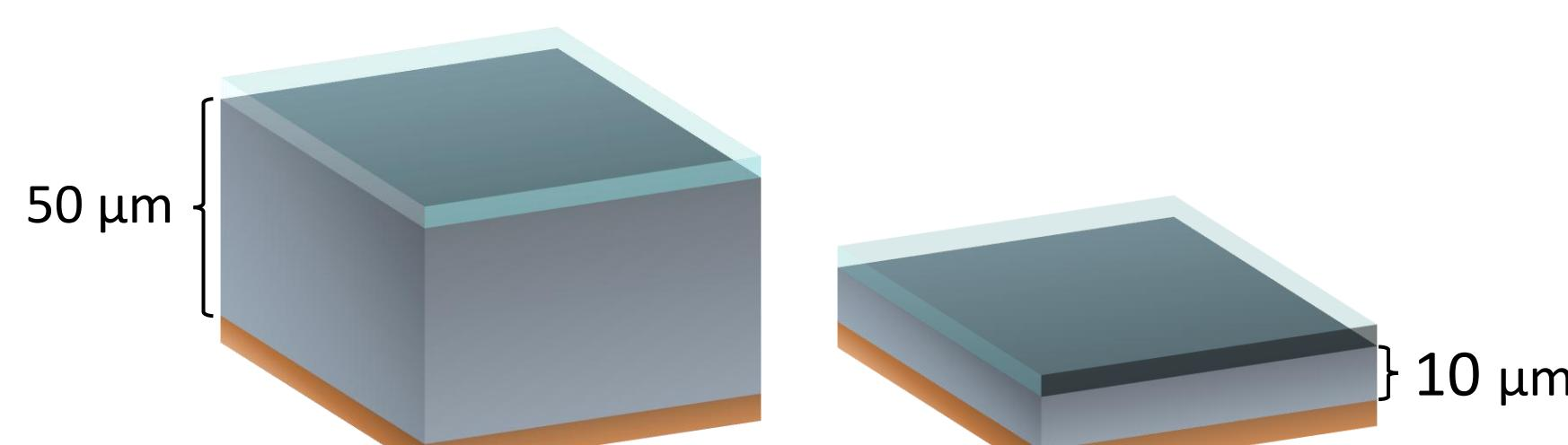
Lithium layer thicknesses of 10  $\mu\text{m}$  and 50  $\mu\text{m}$  were evaluated to represent different application scenarios, including lithium-ion and lithium-sulfur batteries.
